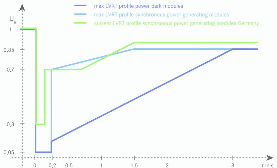
cylinder inlet, and on the responsiveness of the engine controller. Depending on engine size, time spans greater than 100ms are realistic. If the torque is constant and the active power decreases, engine speed will rise. The moment the voltage is recovering, the generator is under-excited, the load angle rises and can reach the transient stability limit for the synchronous machine. In this case, the outcome would be a pole slip which could result in mechanical damage to the synchronous machine.
